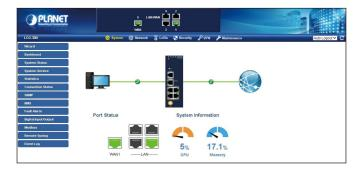
Figure 4-3: Web-based Main Screen of LoRaWAN Gateway
